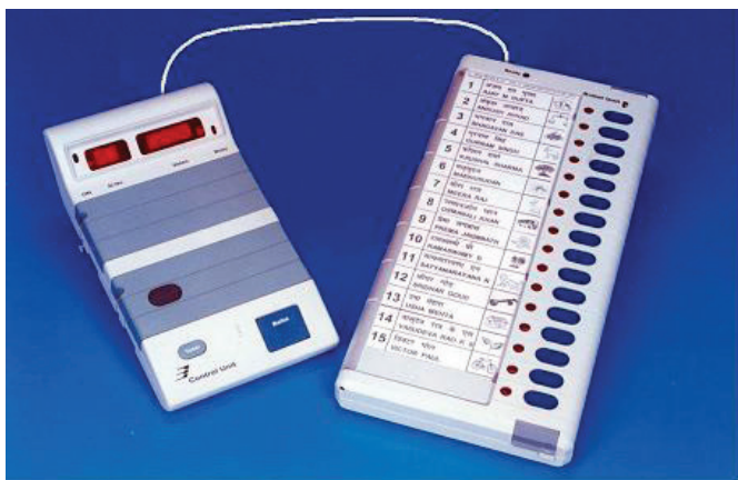
Pic. 4: Electronic Voting Machine: Control Unit on the left and Ballot Unit on the right
